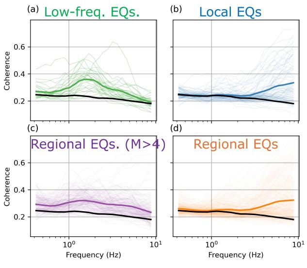
The difficulty of discriminating between Low-frequency earthquakes and large regional earthquakes comes from their similar coherence as a function of frequency.
